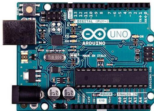
Gambar 1.(a) Board Arduino Uno / ATMEGA 328 Program di Arduino
